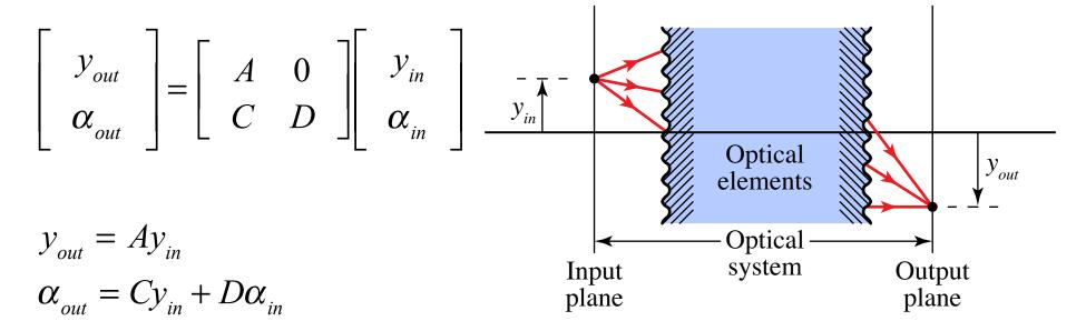
When B = 0, the input and output planes are object and image planes, respectively, and the transverse magnification of the system m = A.
