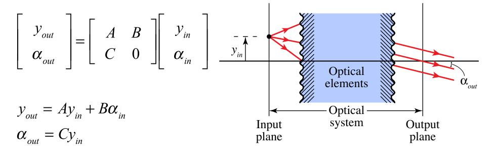
When D = 0, the input plane for the optical system is the input focal plane.
