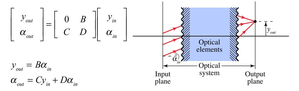
When A = 0, the output plane for the optical system is the output focal plane.
