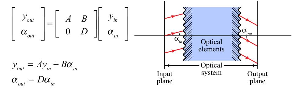
When C = 0, collimated light at the input plane is collimated light at the output plane, but the angle with the optical axis is different. This is a telescopic arrangement, with an angular magnification of  $D = \alpha_{out} / \alpha_{in}$ .
