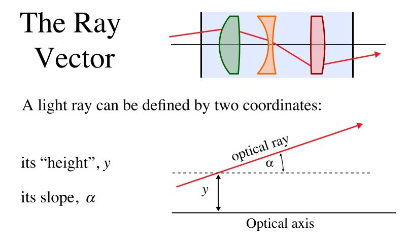
These parameters define a **ray vector**, which will change with distance, and/or as the ray propagates through optical interfaces and elements.
